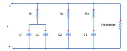
Capacitors  $C_1$ ,  $C_2$ , and  $C_3$  have fixed capacitances. The capacitance of capacitor  $C_v$  depends on the voltage across it. Resistors  $R_1$ ,  $R_2$ , and  $R_3$  have fixed resistances. The voltage across each individual fixed capacitor in the Supercapacitor block is calculated as
