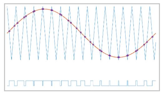
• Asymmetric — Sampling occurs at the upper and lower boundaries of the carrier wave. The comparison occurs at the intersection that follows the sampling.
