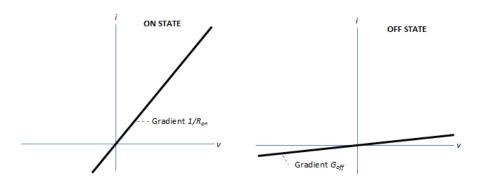
The ideal semiconductor switch is in the on state if the gate-cathode voltage exceeds the specified threshold voltage. Otherwise the device is in the off state.
