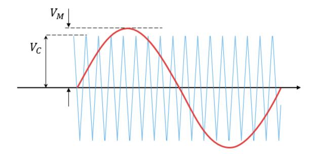
If overmodulation occurs, the output voltage of the power converter clamps to the positive or negative DC rail.
