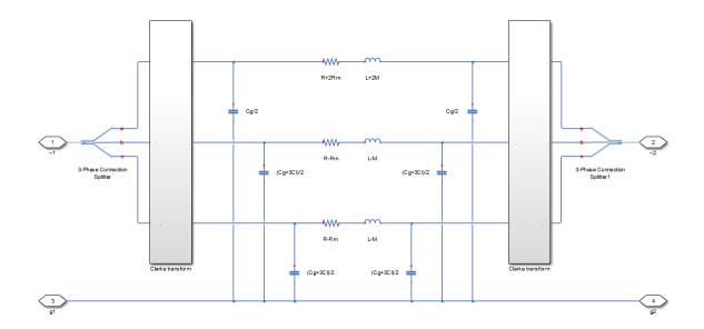
To increase fidelity, you can use the **Number of segments** parameter to repeat the pisection N times, resulting in an N-segment transmission line model. More segments significantly slows down your simulation.
