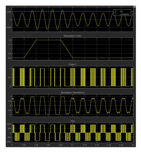
The modulation index is greater than one between 0.03-0.09 seconds. During overmodulation:
