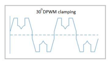
Selecting a positive or negative 30-degree phase shift affects the clamping intervals for 60-degree DPWM.
