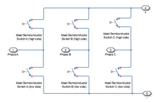
The figure shows the equivalent circuit for a converter with partially controlled switching devices (e.g. thyristors).
