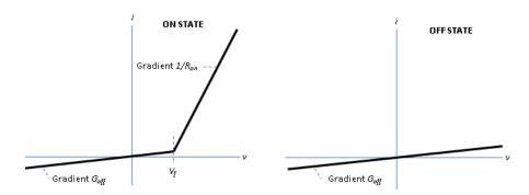
In the on state, the collector-emitter path behaves like a linear diode with forward-voltage drop,  $V_f$ , and on-resistance,  $R_{on}$ .
