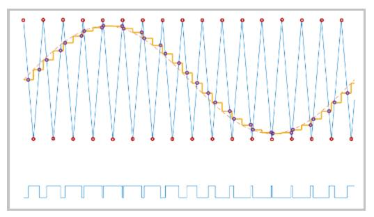
• Symmetric — Sampling occurs only at the upper or the lower boundaries of the carrier wave. The comparison occurs at the intersection that follows the sampling. The figure show upper boundary sampling.
