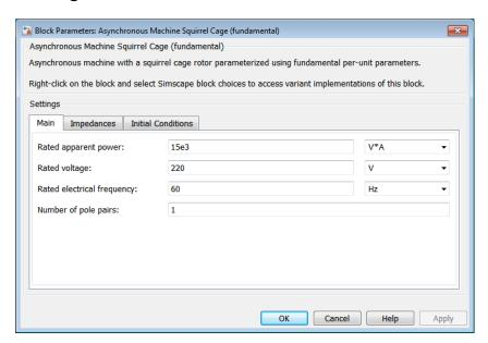
All default parameter values are based on a machine delta-winding configuration.
