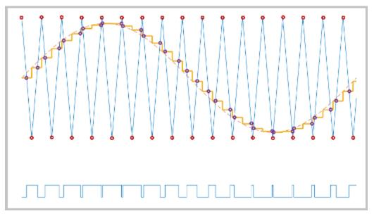
• Symmetric — Sampling occurs at only the upper or the lower boundaries of the carrier wave. The comparison occurs at the intersection that follows the sampling. The figure show upper boundary sampling.
