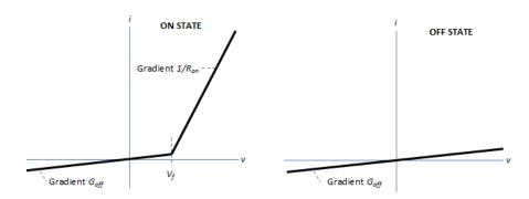
In the on state, the anode-cathode path behaves like a linear diode with forward-voltage drop,  $V_f$ , and on-resistance,  $R_{on}$ .
