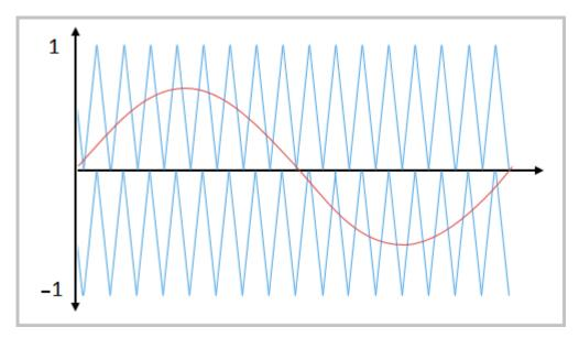
**3** Generates a switch-on pulse if a sample is higher than the carrier signal or a switch-off pulse if a sample is lower than the carrier wave.
