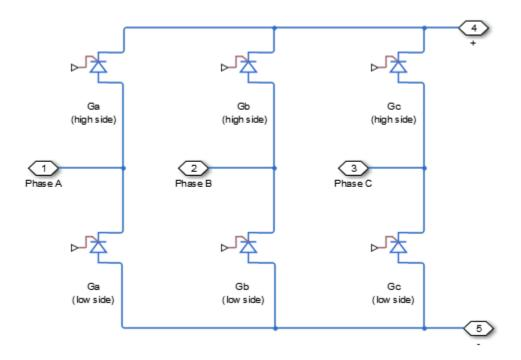
Control the gate ports of the six switching devices via an input to port G on the Converter block:
