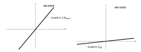
In the on state, the drain-source path behaves like a linear resistor with resistance,  $R_{ds\_on}$ .
