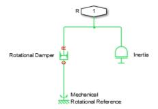
Based on the value you select for the Specify inertia parameterization by parameter, you specify inertia J directly or using the machine inertia constant H.
