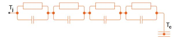
A Foster thermal model contains one or more instances of Foster thermal model elements. The figure shows an equivalent circuit for a Foster thermal model element.
